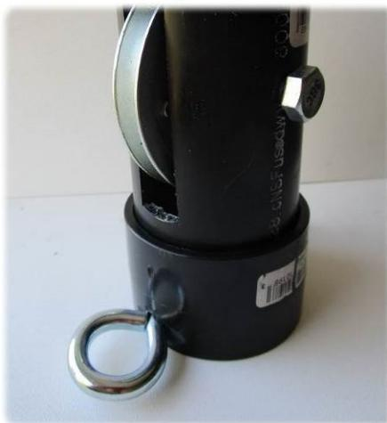
If the assembly is to be mounted at the top of a threaded pipe, drill a 5/16" inch hole through the coupler 7/16" from its top, and inline with the notches.
