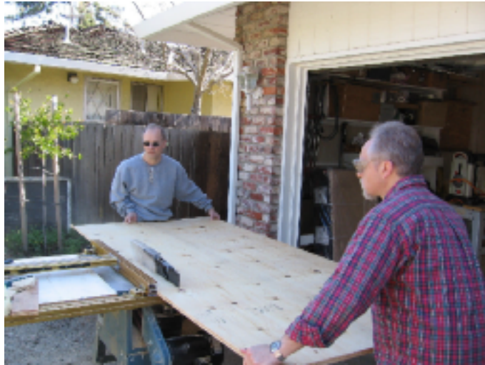
Ripping parts to the desired width on a table saw is the first step.
