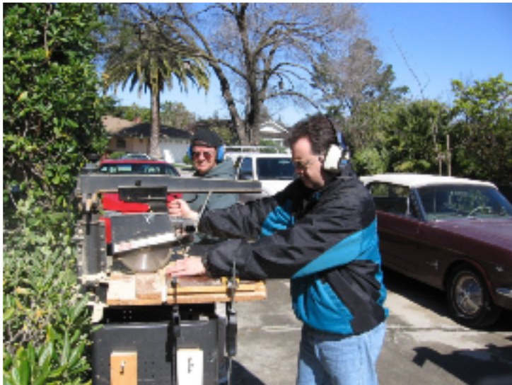
A radial arm saw is used to cut the strips into pieces of the proper length. One person feeds the strips from the right against a stop, and the other operates the saw and removes the piece.
