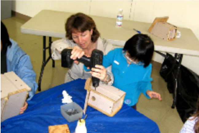
Children can control the speed of the driver if an adult holds the tool. Note how the child's hand fits at the trigger to control the speed of the drill.
