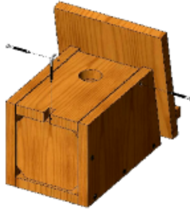
Figure 6. L-screw front closure
