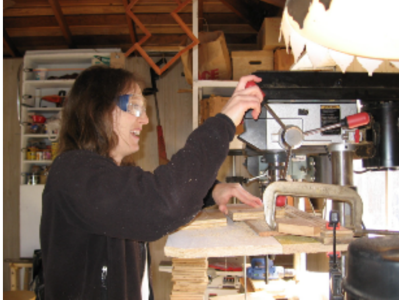
Clamped stops held define equivalent pivot holes on the drill press.
